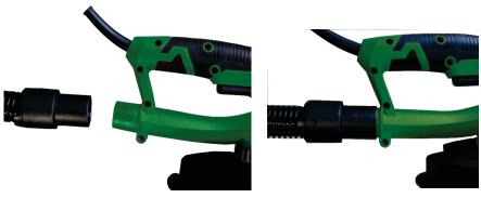
b) Screw the handle onto the side of the sander, as shown below:
